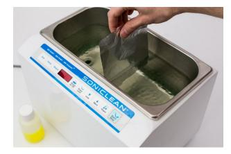
Cut thin aluminium foil (0.025mm) to suitable size for the machine tank.
